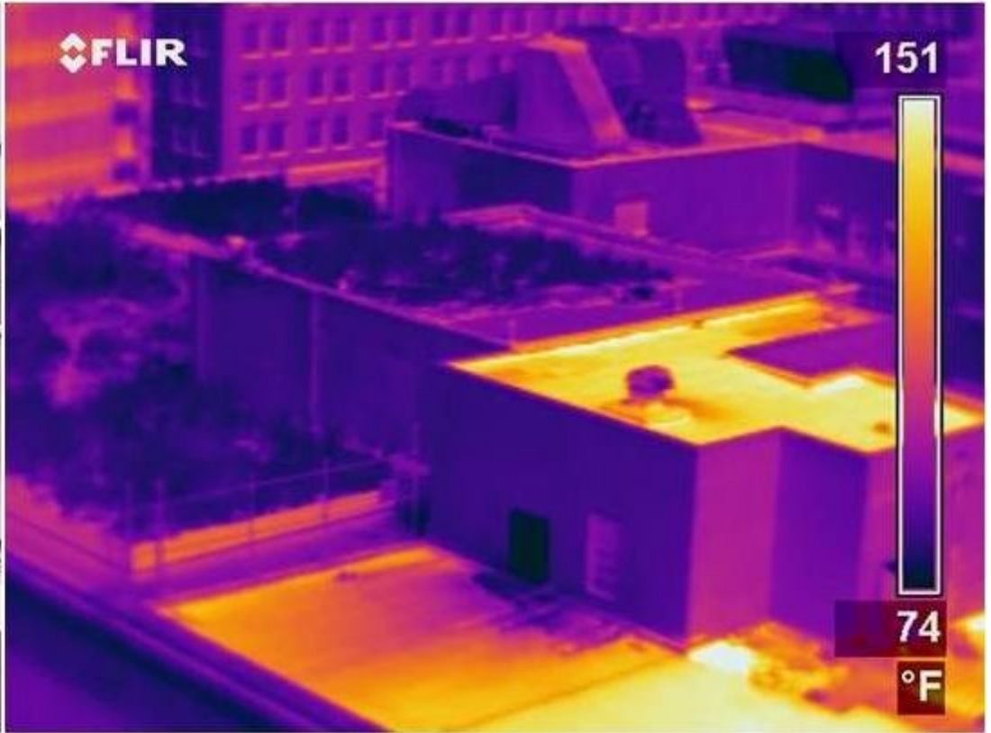
Paul Bamson Architecture : Chicago City Hall (green roof) and Cook County side (conventional roofing).
